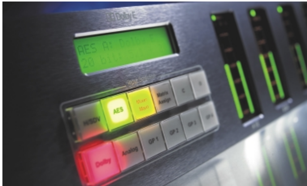
TSL's new AMU2-8HD Dolby audio monitoring unit: 'Among the problems that broadcasters perceive when using Dolby E is that video delay is introduced when you encode and a further delay when you decode; whatever you do with the audio you have to do with the video'
